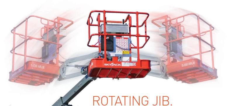
The SJ30 ARJE (Articulating Rotating Jib Electric Boom) offers a working height of 11 m, and horizontal outreach of 6.25 m. Ideal for warehouse, manufacturing and industrial settings that require up and over clearance in tight, confined spaces, the SJ30 ARJE has a width of 1.19 m and up and over clearance of 4 m.
