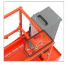
VERTICAL MAST LIFTS Use only on listed models SJ12 A600 000 001+ SJ12 E A601000906 -SJ16 A600 000 001+ SJ20 601000001+ SJ20 E Model A601000906 -Serial Number 140 000 00+ A601999999 140 000 00+ A601999999 50 lb (23 kg) Rated work load on tool tray 500 lb (227 kg) 350 lb (159 kg) Rated work load including tool tray 1 person 1 person 15'7" Wind rating @ 0 mph (0 m/s) 12' (3.66 m) 19' 6" (5.94 m) (4.75 m) 12' Wind rating @ 28 mph (12.5 m/s) 12' (3.66 m) 13' (3.96 m) (3.66 m)
