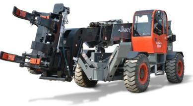
All carriages feature Skyjack's standard 2-Pin Quick Attach design for simple and easy carriage changes. Please see specific telehandler load charts as capacities differ between machines.
