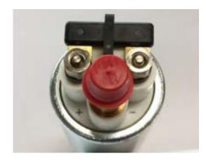
Notice the terminals are marked with positive and negative symbols. *Note: the replacement part will not have darkened symbols.* Verify that the power and ground wires are on the correct terminals or the pump will run backward. Test for good voltage (12V) and a good ground. Make sure there is no rusty or loose connections at the terminals or wire ends.
