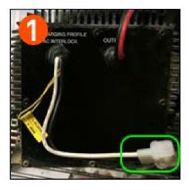
The purpose of the interlock circuit is to prevent the unit from being operated while the charger is plugged in. When the charger is connected to an AC power source, the 120V relay (L1CR) inside the charger opens the contacts cutting power from the main circuit breaker on wire 3A to the 05 wire (power to the emergency stop switch) preventing the machine from operating. See figure 2:
